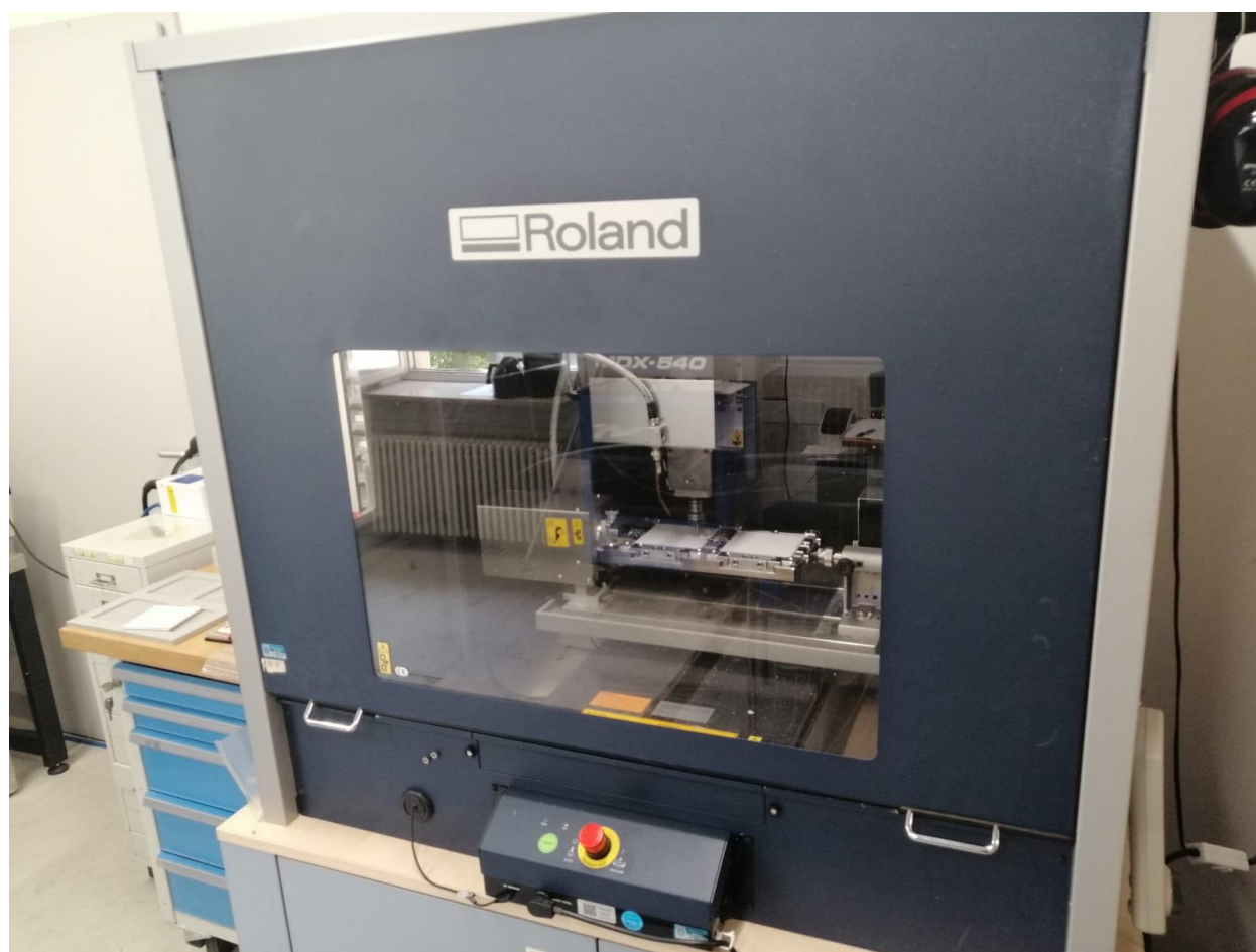
Figure 6. CNC milling machine while milling polycarbonate plates.
