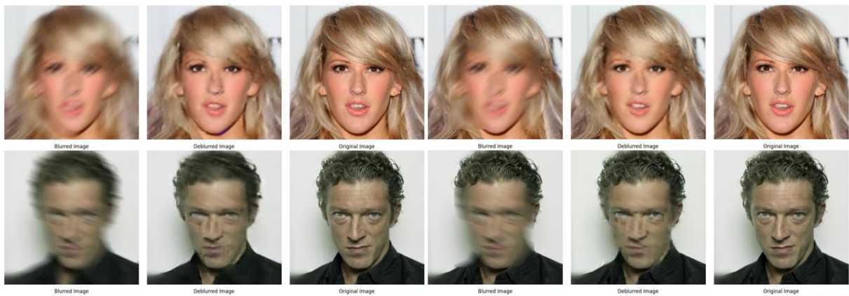
Figure 5.3 Autoencoder model, no segmentation on the left, MediaPipe segmentation on the right
