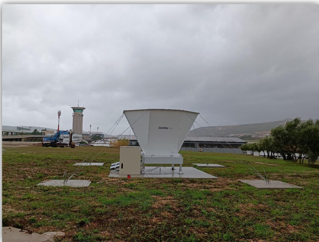
Figure 1 MFAS SODAR at the Split airport.
