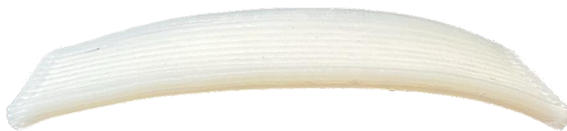
Figure 15 Scaffold after crosslinking
