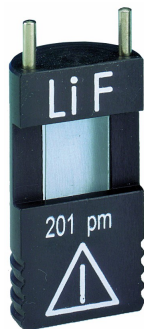
Slika 6.2: Monokristal litijevog fluorida LiF (slika preuzeta s https://phywe.com [13])
