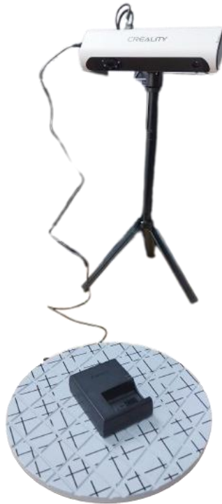
Slika 4.2 – CREALITY CR-Scan 01 3D skener
