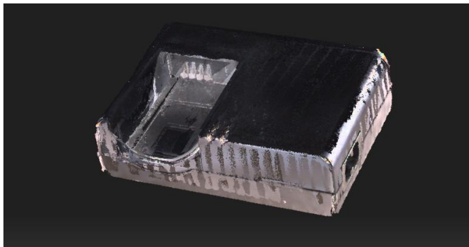
Slika 4.4 – Model skeniran skenerom HP 3D Structured Light Scanner Pro S3
