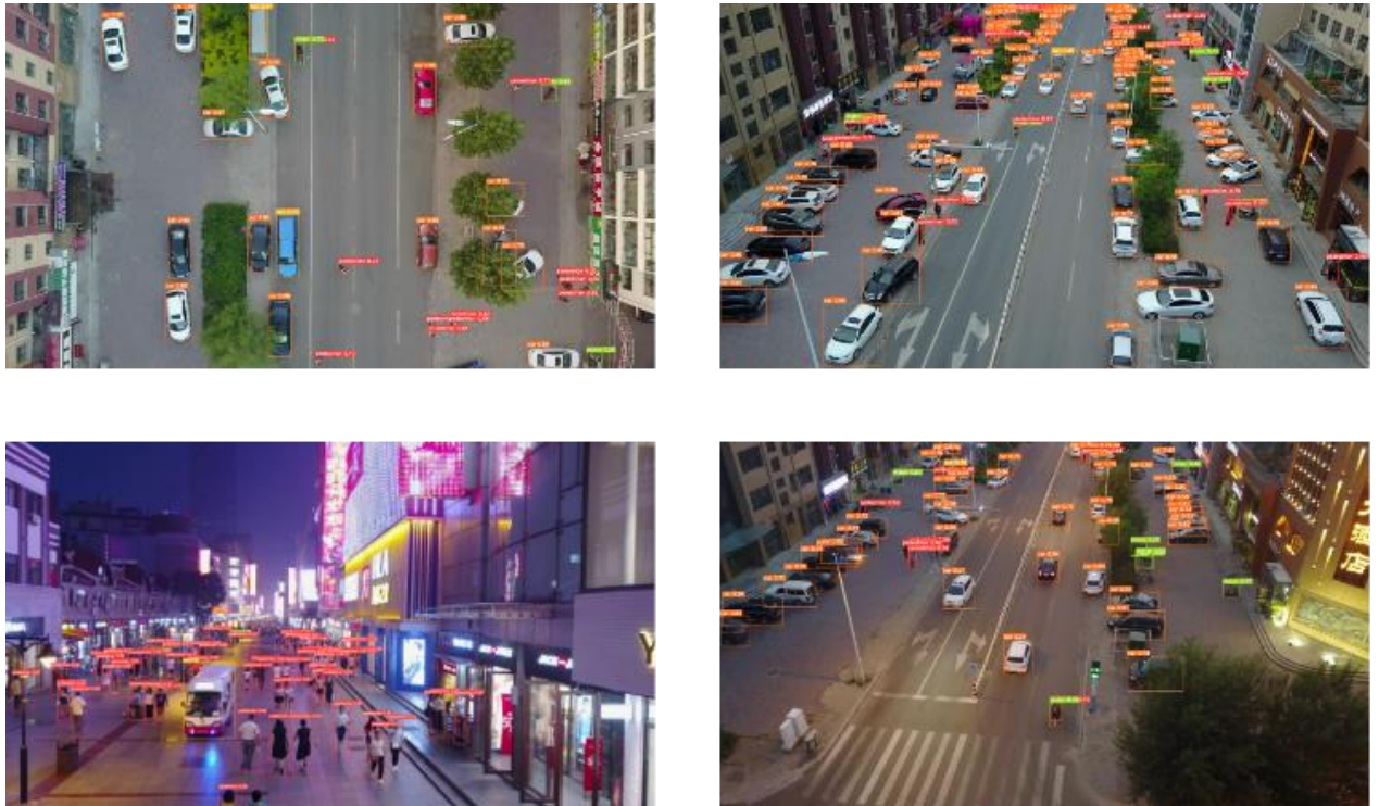
Figure 4.2.4 Predictions on test set images with EL-YOLOv8s which has merged classes.
