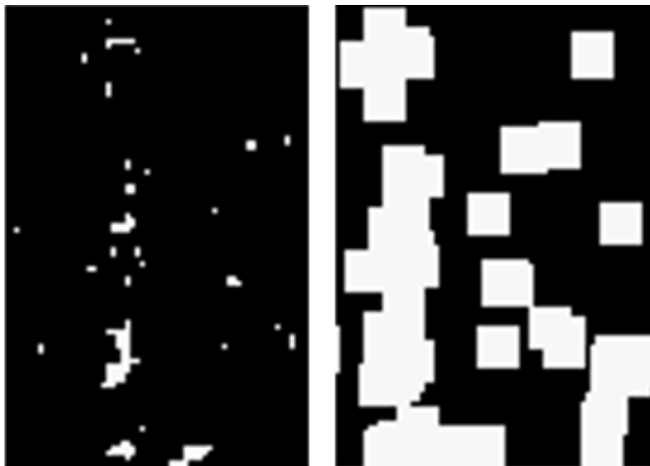
Figure 2.12: Zoomed in view of the remains of an elongated object after erosion (left) and comparison with that same area after dilatation (right).
