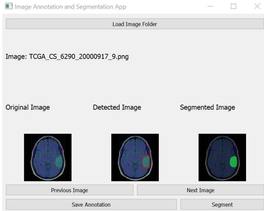
Figure 5.2.4. Display of the original, detected and segmented suspicious images
