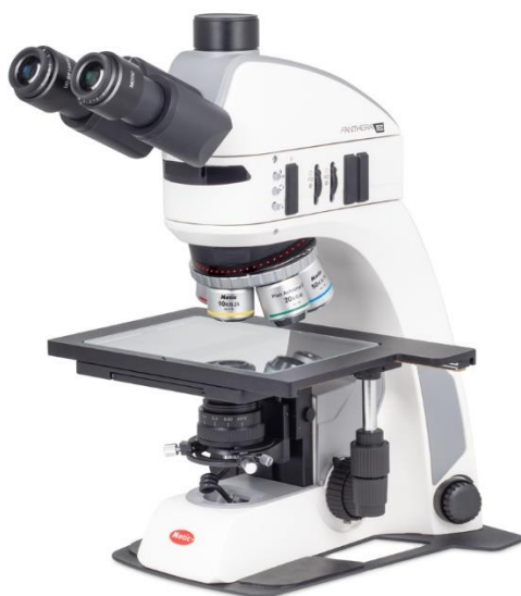
Figure 19 Motic: Panthera TEC MAT BD-T (6x4), microscope with Epi-LED fluorescence attachment 89
