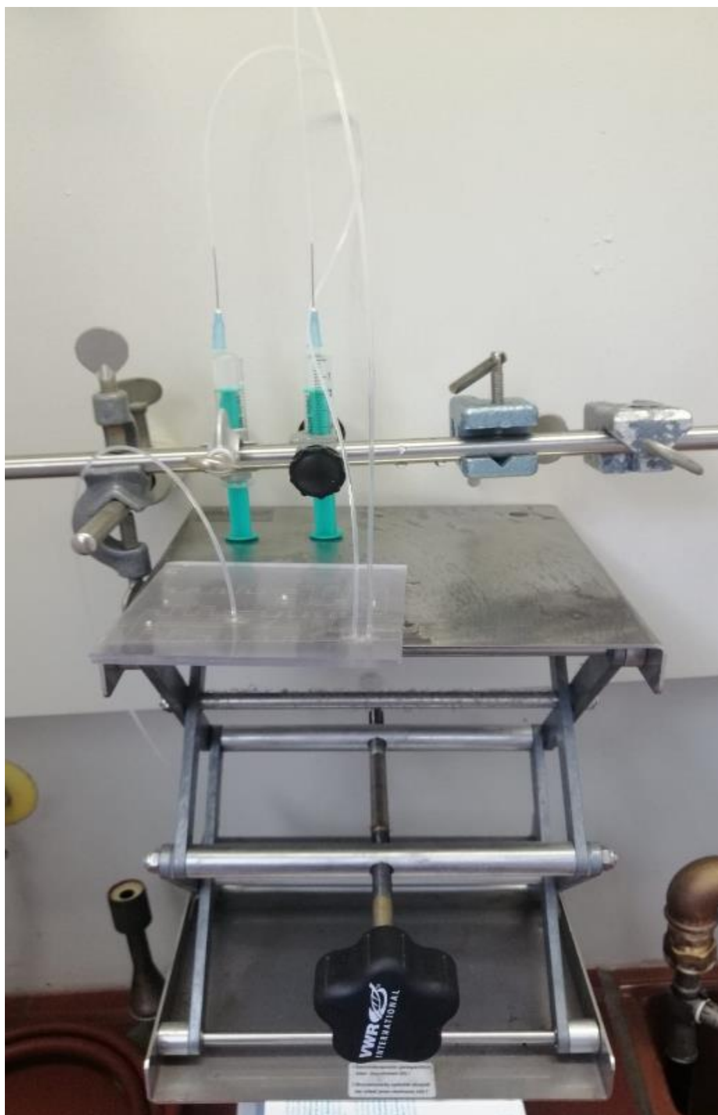
Figure 16. Experimental setup for testing theoretical calculation of microfluidic chip.
