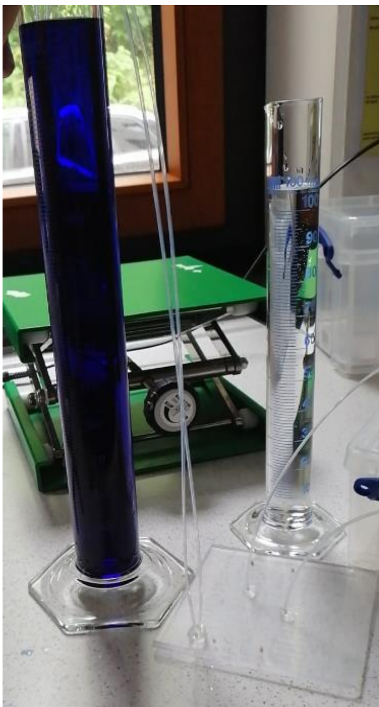
Figure 15. Testing microfluidic chip using hydrostatic pressure. The water was used with blue dye.
