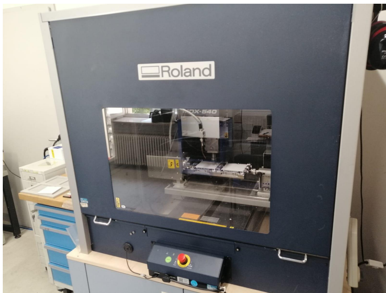
Figure 6. CNC milling machine while milling polycarbonate plates.
