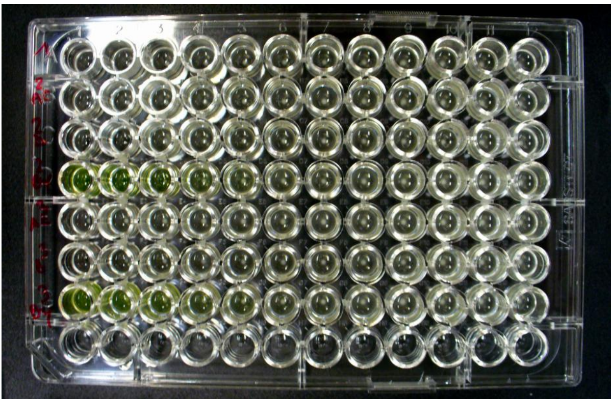
Figure 26. Example of MIC results for S. aureus all ADPs; rows: ADP1, ADP2(AM), [\text{ADP2}]_2 , ADP2(BY), ADP3(AM), [\text{ADP3}]_2 , ADP3(BY), empty; columns: 1 st – 11 th peptide + bacteria + MH starting with concentration 128 \mu\text{M} and decreasing by two-fold dilution method, 12 th negative control = bacteria + MH; white dots on the bottom of the well is grown bacteria.
