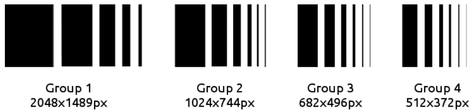
Figure 2.8: How resizing affects line width and intensity.
