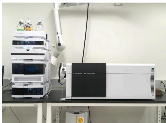
Slika 7. HPLC-MS sustav za analizu. Preuzeto s Biodiscovery Institute. https://bdi.unt.edu/bioanalytical-facility/about/instrumentation .
