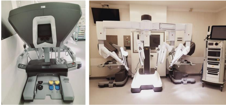
Slika 1 Prikaz robotske konzole i robotskih ruku (Hughes i sur., (2023), The Availability, Cost, Limitations, Learning Curve and Future of Robotic Systems in Urology and Prostate Cancer Surgery)
