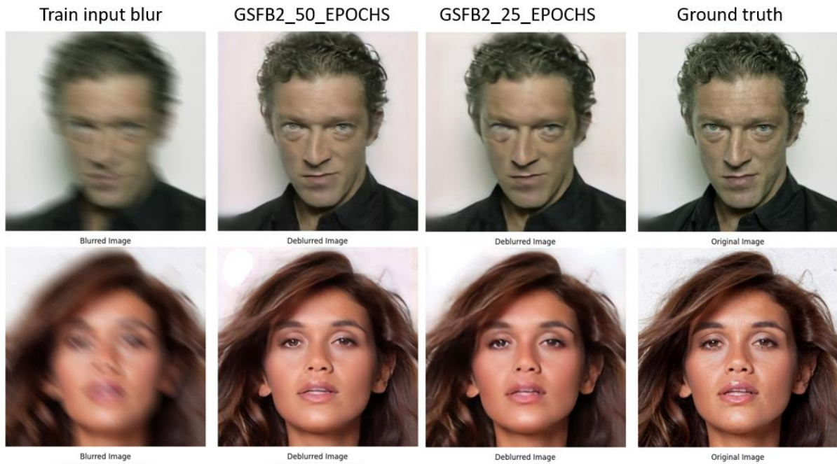
Figure 5.13 Comparison of GSFB2 model trained for 25 and 50 epochs
