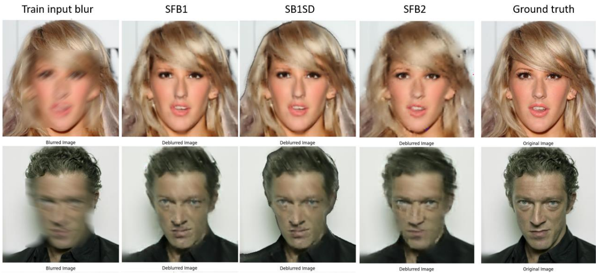
Figure 5.7 ASB2SM model deblurring visual performance on other test datasets
