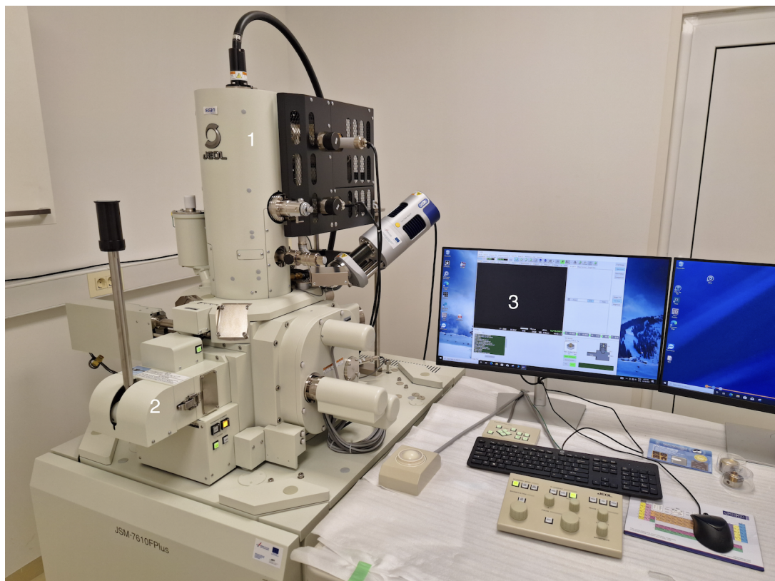
Figure 1: Field Emission Scanning Electron Microscope, JEOL JSM-7610FPlus, used in our research. Primary components are labeled as follows: (1) electron column, (2) sample chamber, (3) computer control system.
