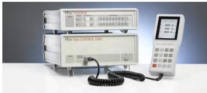
Slika 9. Elektrometar TANDEM Dual Channel (Preuzeto s <http://ptwdosimetry.com> [10])
